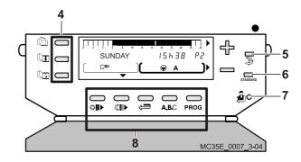
4 Key for access to setting and measurements
