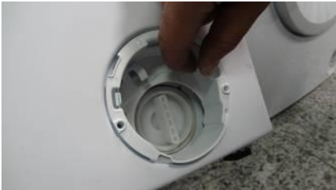
7. Remove the pump cover housing as it is shown in the picture.
