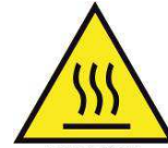
CAUTION HOT SURFACE Caution hot surface
