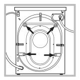
3. Remove the four protective screws and the rubber bush with the respective spacer, situated on the rear of the appliance (see also the installation leaflet).
