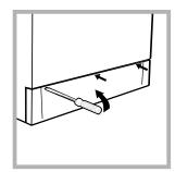
using a screwdriver, remove the cover panel on the lower front of the Washer-dryer (see figure);
